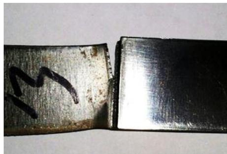
**Figure 2:** Failure across tensile shear testing load
