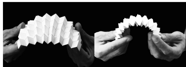
Fig 2.1 Mechanical Behavior of Egg box sheet
