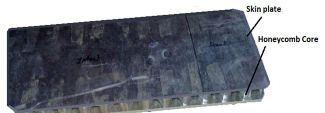
Fig.8 Specimen of Honeycomb Structure
