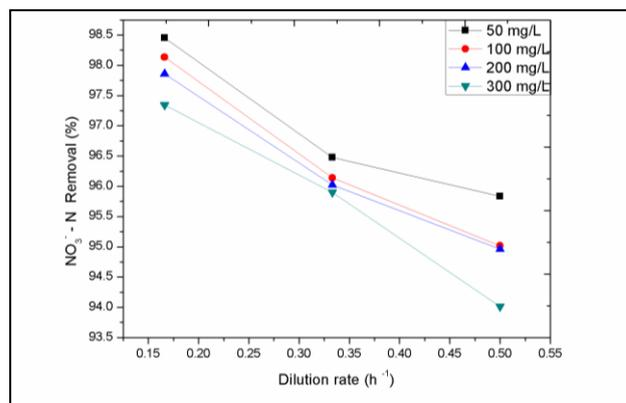
**Fig.3:** Effect of dilution rate at different influent nitrate concentration on percentage nitrate removal at steady state for GAC loading 40 gm
