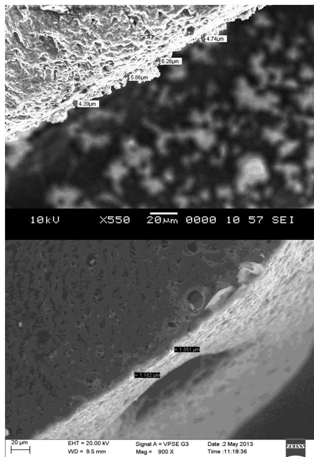
Fig.7: SEM Pictures of biofilm on Granular activated carbon
