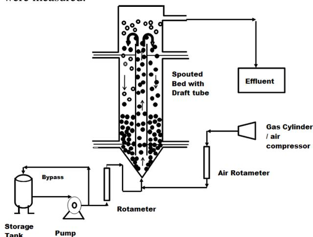
**Fig.1 (b):** Experimental setup of Draft Tube Spouted Bed Bioreactor
