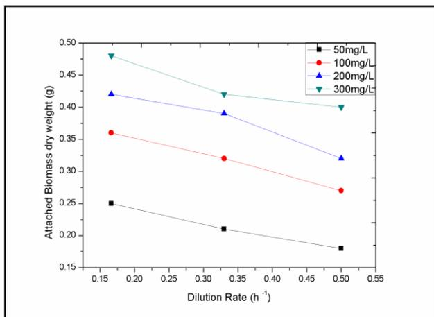
Fig. 5: Effect of Dilution rate on attached biomass for different influent nitrate concentration at steady state
