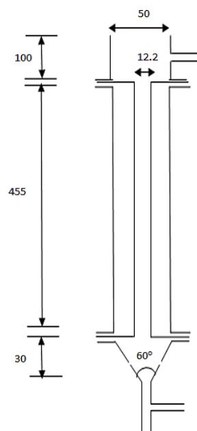
**Fig.1 (a):** Schematic diagram of Draft tube Spouted Bed Bioreactor
