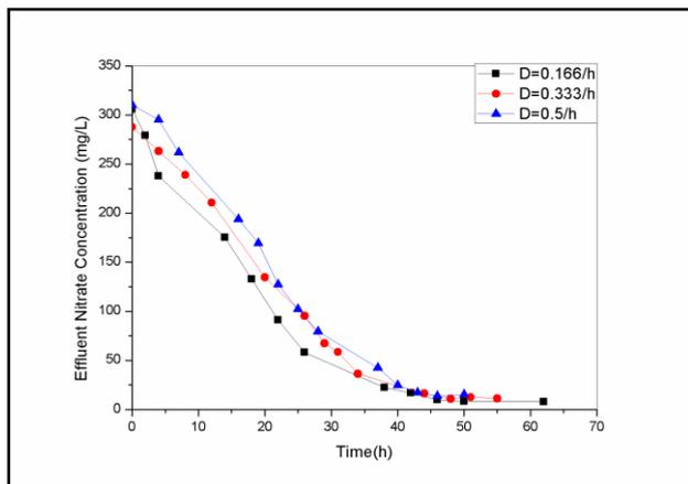
**Fig.2:** Effect of dilution rate on effluent nitrate concentration during start up for different influent nitrate concentration (a):50 mg/L (b): 100mg/ L (c): 200 mg/L (d): 300 mg/L
