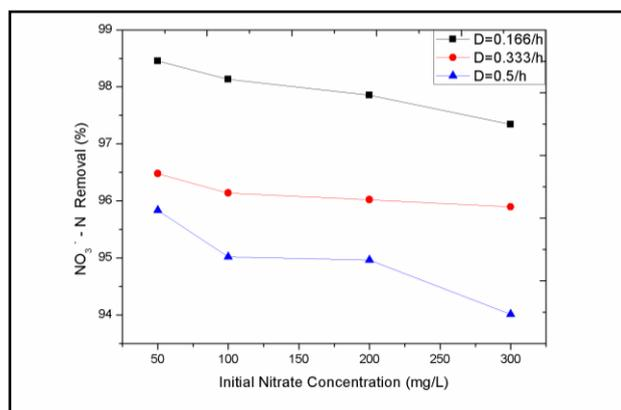
**Fig.4:** Effect of influent nitrate concentration at different dilution rates on percentage nitrate removal at steady state
