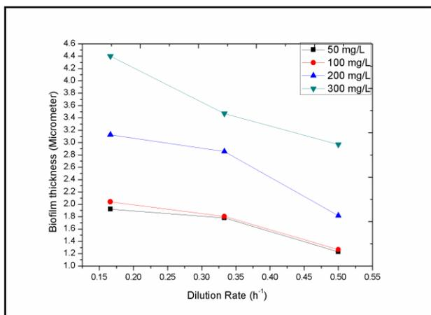
Fig. 6: Effect of dilution rate on biofilm thickness for different influent nitrate concentration at steady state
