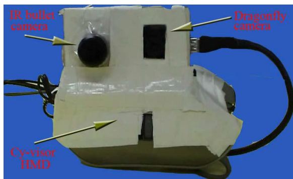
Fig. 2: Capture and Visualization System for Invisible Marker Based Augmented Reality system.
