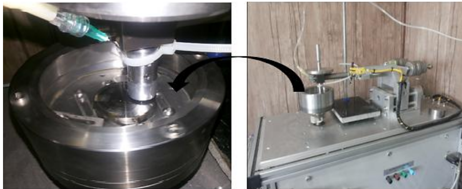
Fig. 2 Wear test apparatus
