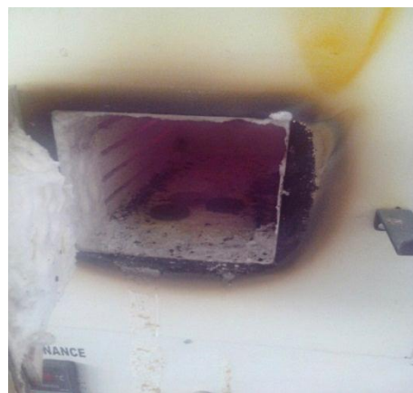
Fig 3: Slow Cooling of Specimens in Furnace
