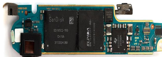
Fig.5 The main logic board of Google glass
