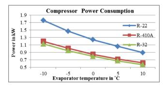
Figure 8 Power consumption for different refrigerants
