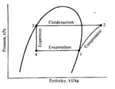
Figure 4.P, h Diagram for refrigeration cycle
