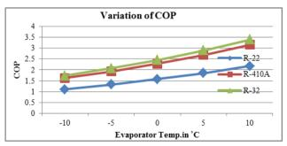
Figure 6 Variation of COP with evaporator
