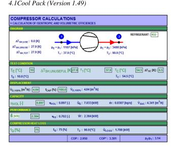
Figure 5 Simulation of Air conditioning Compressor
