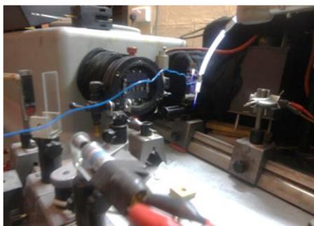
**Fig.2:** Measuring the spectra by monochromator with photomultiplier
