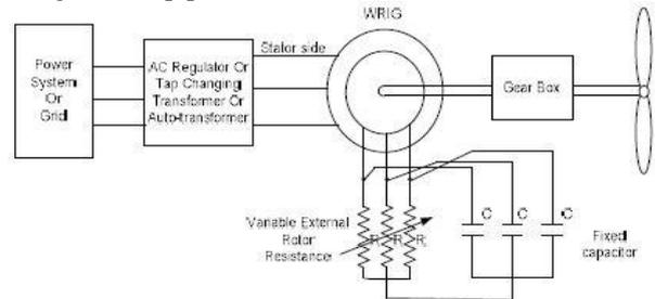
**Fig. 5** Circuit topology of the combined input voltage and slip power control with fixed capacitor scheme
