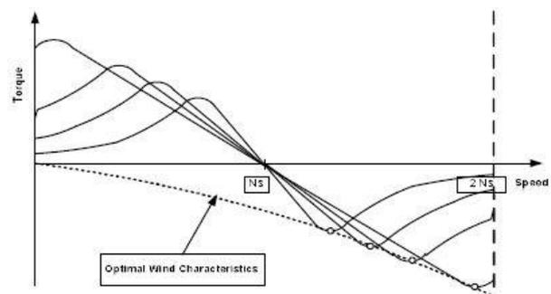
**Fig. 4** Characteristics of a WRIG with rotor resistance as well as stator voltage control
