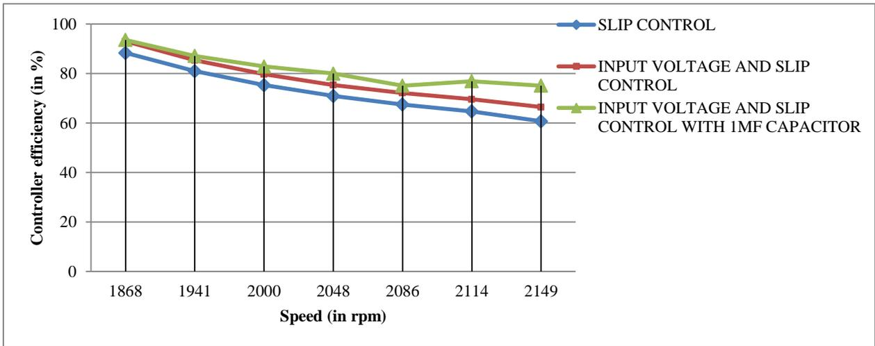
Fig.10 Efficiency versus speed
