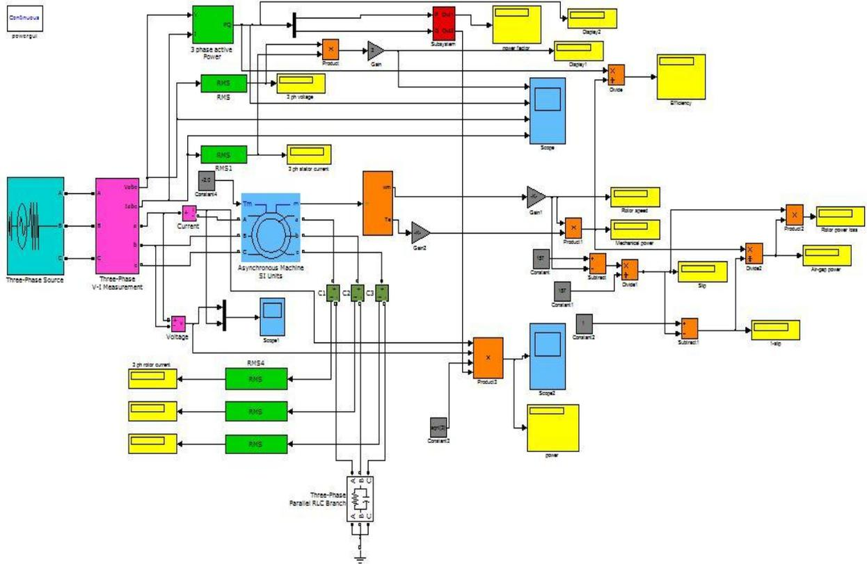
Fig.6 MATLAB Simulation model of WRIG feeding power to grid
