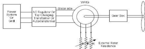
**Fig. 3** Circuit topology of the combined input voltage and slip power control scheme
