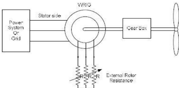
**Fig. 1** Rotor resistance control of a wound rotor induction generator
