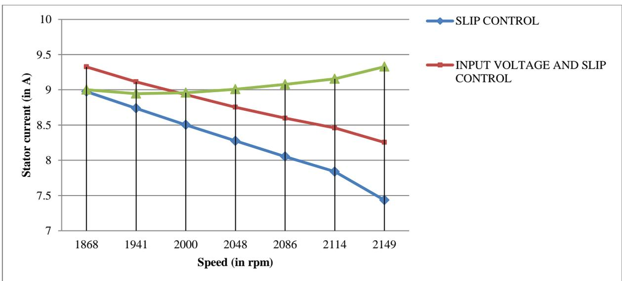
Fig.12 Stator current versus speed
