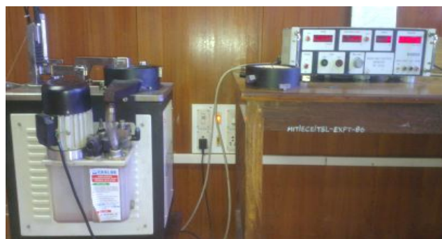
Figure 2.3 Experimental setup for Wear test on Pin on Disc
