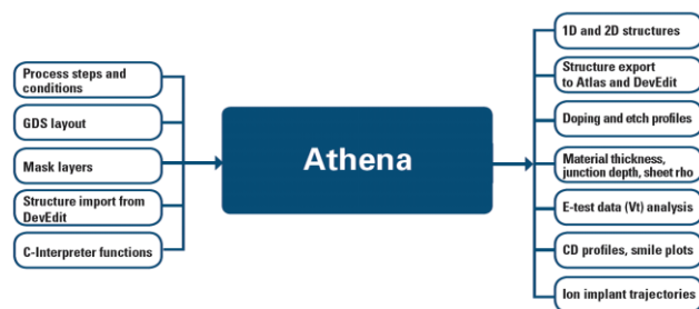
Fig.2 Athena Input and Output Block diagram
