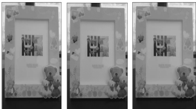
Fig.5 Reconstruction by opening and closing (a) sobel (b) prewitt (c) laplacian
