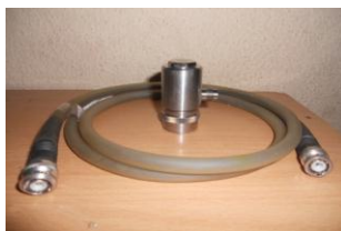
Fig. 3 Magnetic Base vibration pickup
