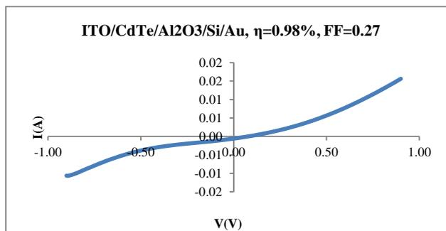
**Figure (7):** I-V curve of light current for ITO/CdTe/Al<sub>2</sub>O<sub>3</sub>/Si/Au device in which the thickness of Al<sub>2</sub>O<sub>3</sub> is 3.5nm
