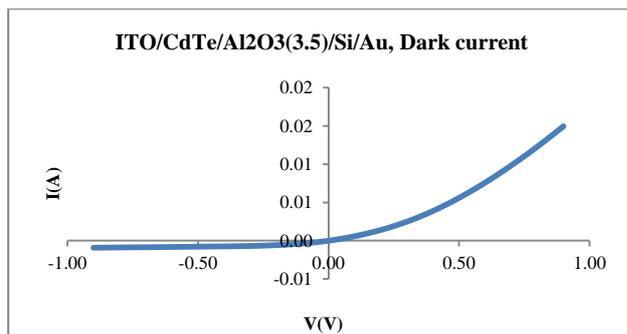
**Figure (6):** I-V curve of dark current for ITO/CdTe/Al<sub>2</sub>O<sub>3</sub>/Si/Au device in which the thickness of Al<sub>2</sub>O<sub>3</sub> is 3.5nm
