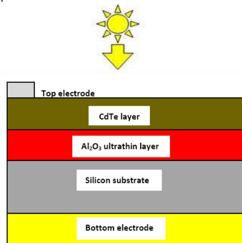
**Figure 1:** Schematic view of the prepared solar cell
