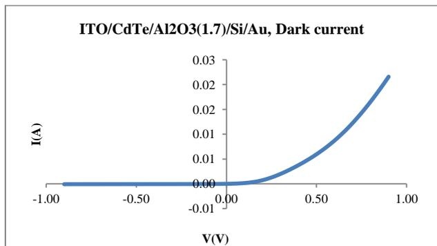
**Figure (4):** I-V curve of dark current for ITO/CdTe/Al<sub>2</sub>O<sub>3</sub>/Si/Au device in which the thickness of Al<sub>2</sub>O<sub>3</sub> is 1.7nm
