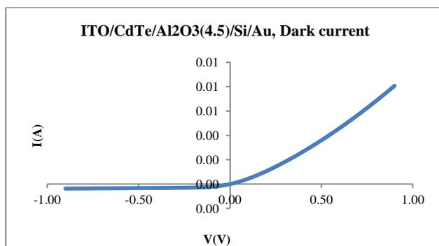
**Figure (8):** I-V curve of dark current for ITO/CdTe/Al<sub>2</sub>O<sub>3</sub>/Si/Au device in which the thickness of Al<sub>2</sub>O<sub>3</sub> is 4.5nm
