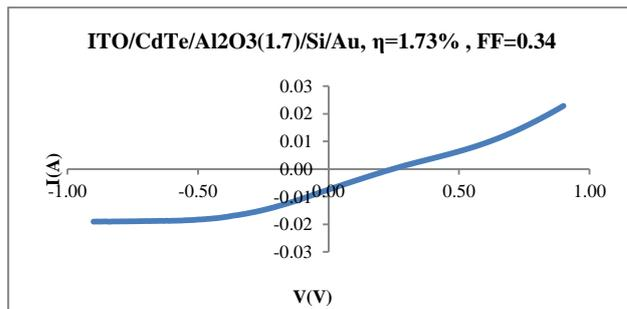
**Figure (5):** I-V curve of light current for ITO/CdTe/Al<sub>2</sub>O<sub>3</sub>/Si/Au device in which the thickness of Al<sub>2</sub>O<sub>3</sub> is 1.7nm
