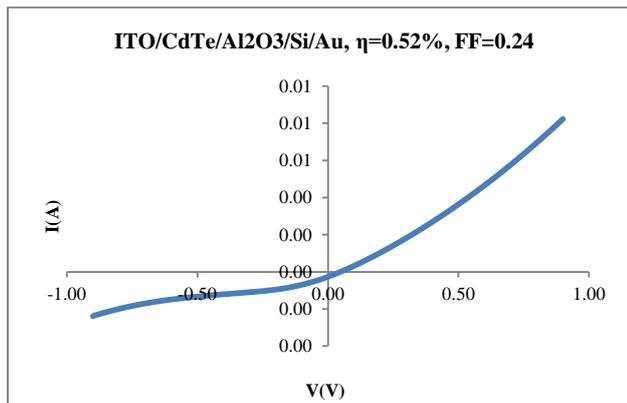
**Figure (9):** I-V curve of light current for ITO/CdTe/Al<sub>2</sub>O<sub>3</sub>/Si/Au device in which the thickness of Al<sub>2</sub>O<sub>3</sub> is 4.5nm
