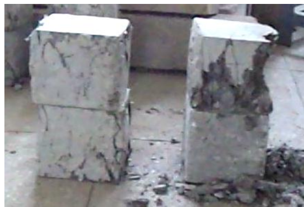
Fig.4 Failure of a specimen of HFR & plain concrete under compressive strength test.
