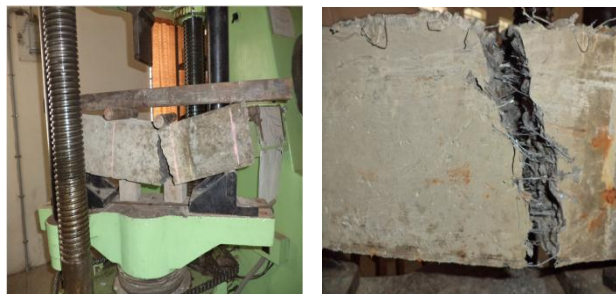
(a) Plain Beam (b) HFRC Beam
