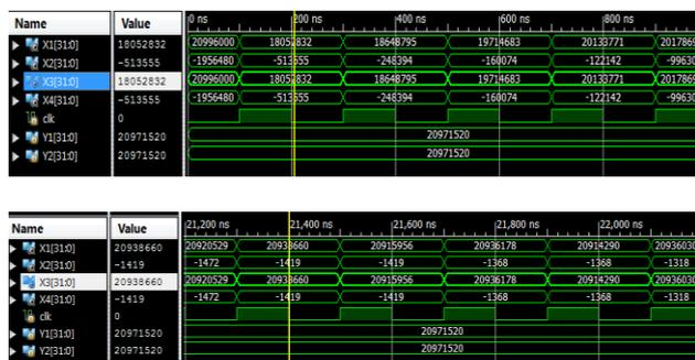
**Figure 19** Simulation result of parallel kalman filter
