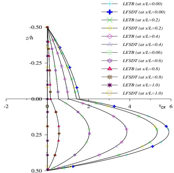
**Fig 3:** Variation of transverse shear stress ( $\tau_{zx}^{EE}$ ) through the thickness of cantilever beam subjected to sinusoidal load and obtained using equilibrium equations for aspect ratio 4
