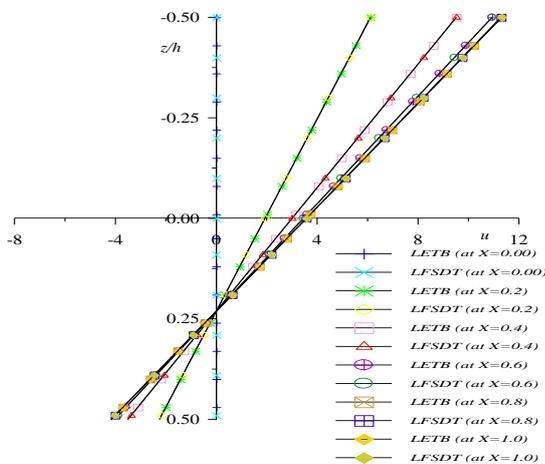
**Fig. 1:** Variation of axial displacement (u) through the thickness of cantilever beam when subjected to sinusoidal load for aspect ratio 4
