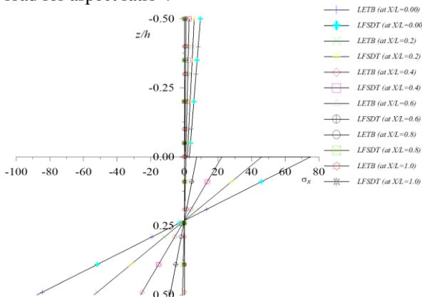
**Fig 2:** Variation of axial stress ( $\sigma_x$ ) through the thickness of cantilever beam when subjected to sinusoidal load for aspect ratio 4
