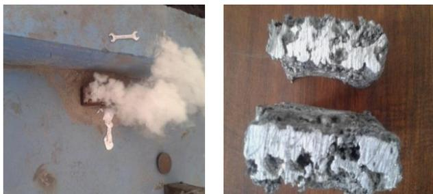
Fig 2.1. Production of open cell aluminium foam.
