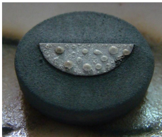
Fig.2(a): Blistering at the ceramic surface
