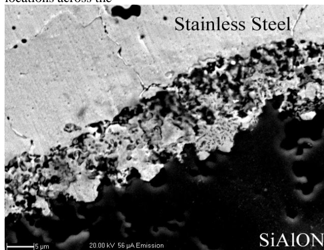
Fig.3 (b): electron micrograph of \alpha -SiAlON-316 stainless steel interface prepared under hot pressing. Some pores are indicated by arrows on the interface at steel side.
