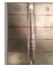
Fig.1 Butt welded specimen prepared by GTAW
