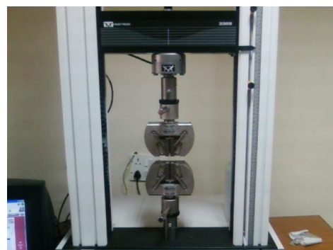
Fig.2 A 50kN UTM table top facility at DTU
