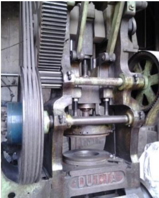
Fig. 2 Mechanical press used in deep drawing process
