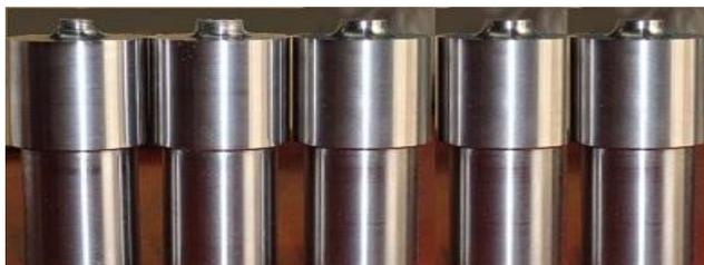
**Fig.2** Fabricated FSW tools
