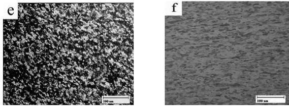
**Fig. 8:** Microstructure of weld nugget zone (a) concave shoulder taper cylindrical threaded pin with radius 3mm (b) concave shoulder taper cylindrical threaded pin with radius 3.5mm (c) concave shoulder taper cylindrical threaded pin with radius 4mm (d) straight cylindrical threads with radius of curvature 3mm and (e) straight cylindrical threads with radius of curvature 3.5mm (f) Microstructure of AA2014-T6 base material
