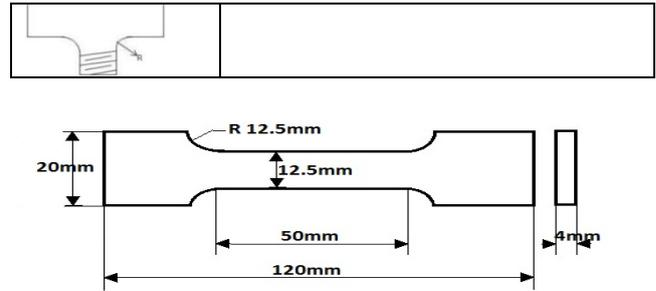
Fig. 4(a). Tensile test specimen standard dimension
