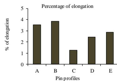
Fig.5. Comparing the various pin profiles and Mechanical properties; (a) UTS and pin profiles, (b) yield strength and pin profiles, and (c) % of elongation and pin profiles.
