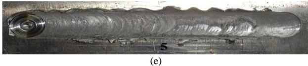
Fig. 3 (a), (b), (c) Welds are formed by using threaded taper concave cylindrical pin with R= 3.0 mm, R = 3.5 mm and R = 4.0 mm. (d) And (e) welds are formed by using threaded taper straight cylindrical pin with R = 3 mm and R= 3.5 mm.
