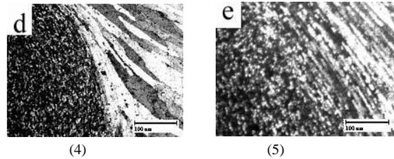
**Fig.9:** Microstructures in weld nugget-TMAZ interface (1) welded by friction stir tool A (2) welded by friction stir tool B (3) welded by friction stir tool C (4) welded by friction stir tool D (5) welded by friction stir tool E.
