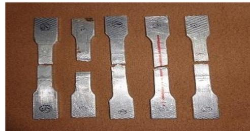
Fig.4(b). Specimen after tensile testing
