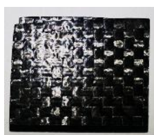
Fig. 2 Workpiece Material (Carbon Fiber Epoxy Composites)
