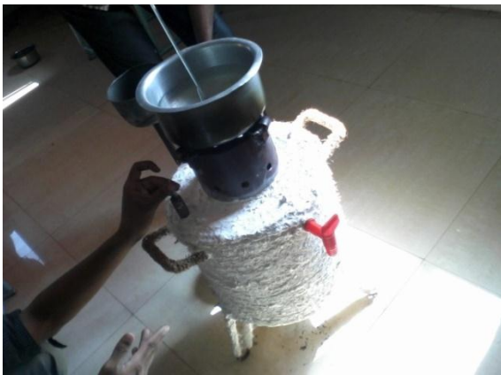
Fig 2: Water boiling test
