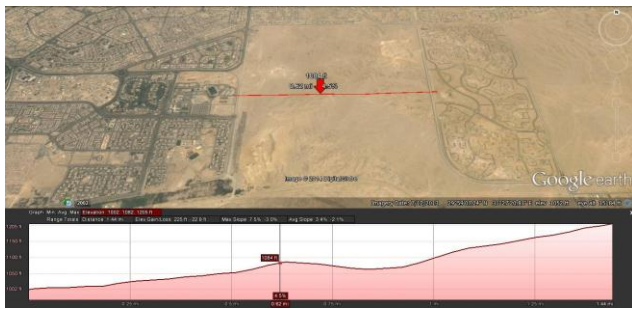
Figure 7 shows a cross-section of the Reservation from east to west.
