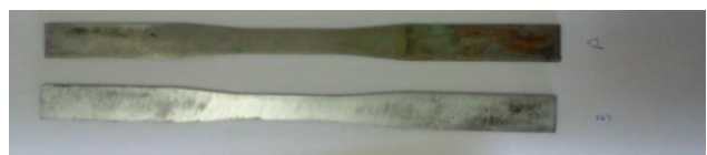
Fig.3 Aluminium with and without nickel coated
