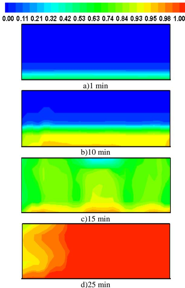
**Fig. 3.** Liquid Fraction contours for different time in the PCM unit.
