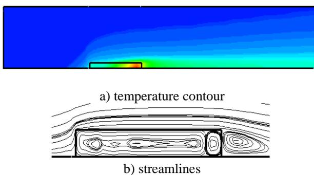
**Fig. 4.** Streamline and temperature contour for  $q''=1000$  w/m<sup>2</sup> and  $h_p=0.25$ cm after 25 min
