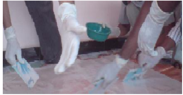
Fig.3 Wetting the cloth with matrix (resin & hardener)
