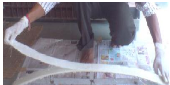
Fig.5 Laying the wetted cloth on mould
