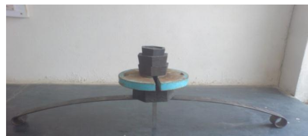
Fig.9 Static load on master leaf of metallic leaf spring
