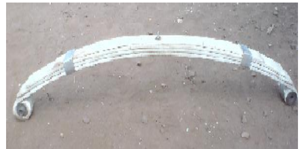
Fig.7 Finished component (composite leaf spring)
