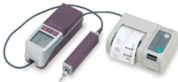
Figure 2: Mitutoyo SJ-201P Profilometer
