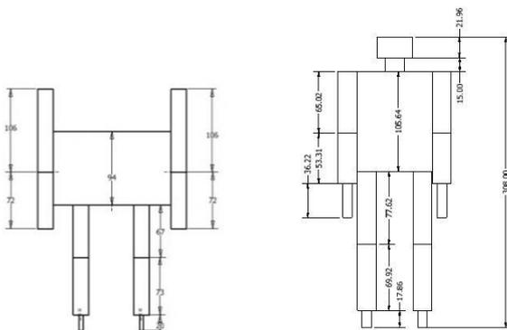
Fig.3 Comparison of Parinat-1 dimensions with actual human body segments
