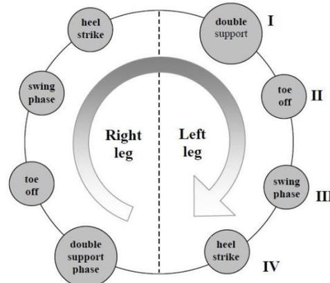
Fig.8 The cyclic phase rotation of biped walking
