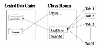
The architecture can be divided into two components; the CENTRAL DATA CENTER and the CLASSROOM. A Wi-Fi connection is needed in every class. Here TAB 1 to TAB N represents the tablets of the students. Marking of the attendance will be controlled by the teacher.
