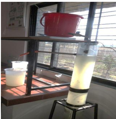
Figure 1: Laboratory scale Compact Jet Loop Reactor
