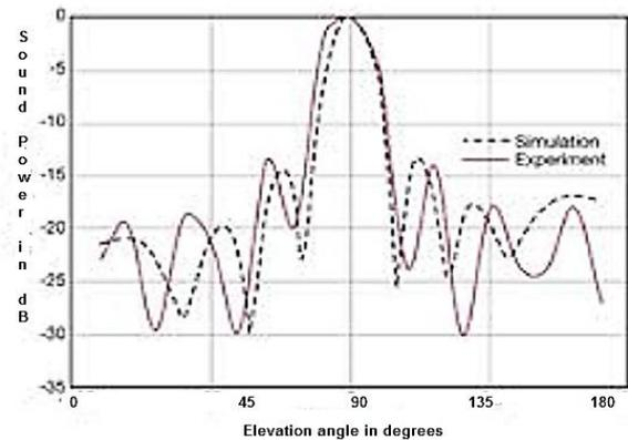
**Figure 3:** Radiation pattern of the uniform 8 x 8 tweeter array antenna at two frequency steps 2 kHz and 2.1 kHz.
