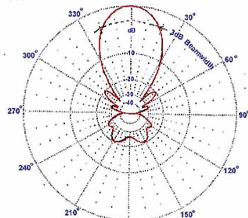
**Figure.5:** Polar radiation pattern for a tweeter at 4.5 kilo Hertz.
