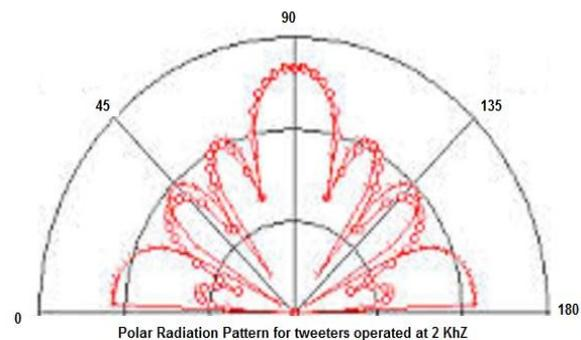
**Figure.4:** Normalized polar Radiation pattern of the uniform 8 x 8 tweeter array antenna at three frequency steps 2 kHz.
