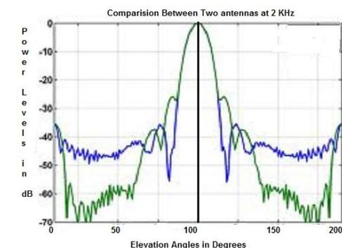
**Figure.6:** Normalized Radiation pattern of the uniform 8 x 8 tweeter array antenna at three frequency steps 2 kHz, and 4. KHz.
