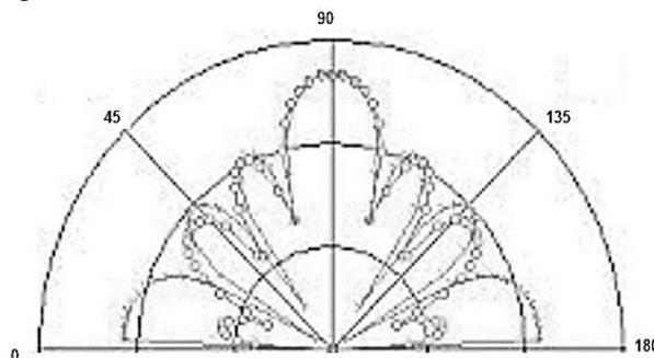
**Figure.8:** Normalized polar Radiation pattern of the uniform 8 x 8 Ahuja array antenna at three frequency steps 4.5 kHz, 4.6 kHz and 4.7 kHz.
