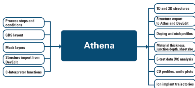
Fig.1 Athena Input and Output Block diagram
