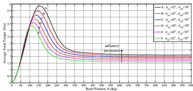
Fig. 10 Average total torque versus rotor position for advance turn-on
