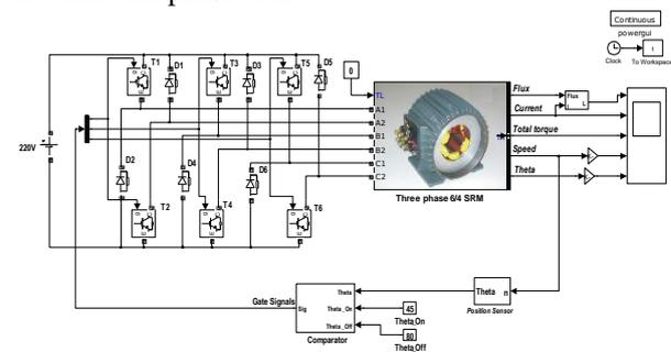
Fig. 2 Simulink model using angle control for 3-ph 6/4 SRM at no-load
