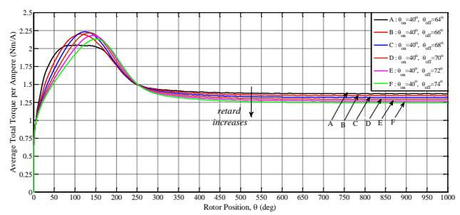
Fig. 15 Average torque per ampere versus rotor position for retard turn-off
