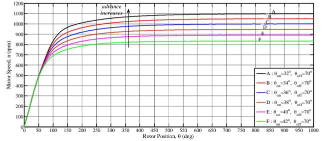
Fig. 12 Motor speed versus rotor position for advance turn-on
