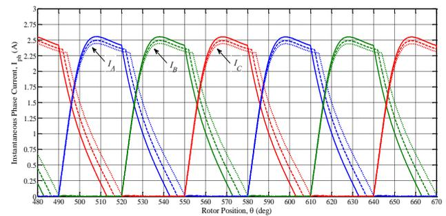
**Fig. 6** Instantaneous motor phases current versus rotor position for retard turn-off
