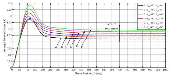
Fig. 13 Average source current versus rotor position for retard turn-off
