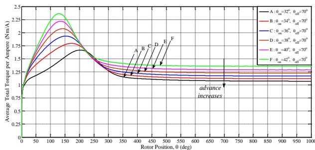
Fig. 11 Average total torque per ampere versus rotor position for advance turn-on
