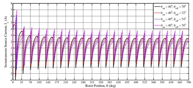
**Fig. 7** Instantaneous source current versus rotor position for retard turn-off
