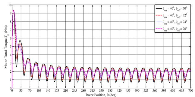
**Fig. 8** Motor total torque versus rotor position for retard turn-off
