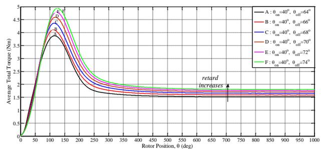
Fig. 14 Average total torque versus rotor position for retard turn-off
