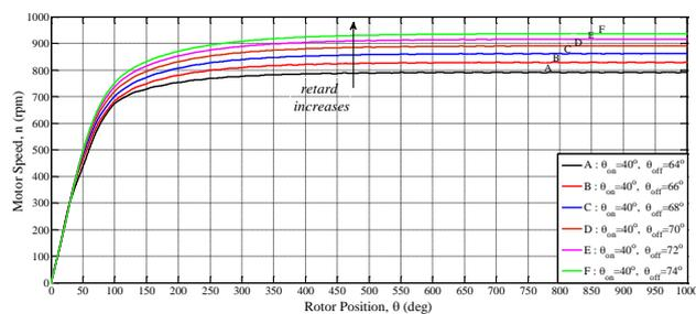
**Fig. 16** Average motor speed versus rotor position for retard turn-off
