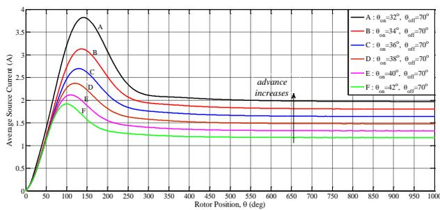
Fig. 9 Average source current versus rotor position for advance turn-on
