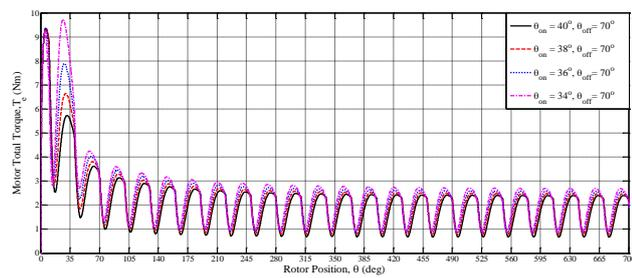
**Fig. 5** Motor total torque versus rotor position for advance turn-on
