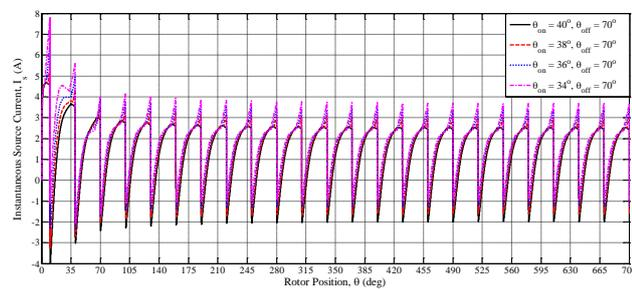
**Fig. 4** Instantaneous source current versus rotor position for advance turn-on
