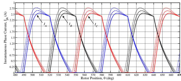
**Fig. 3** Instantaneous motor phases current versus rotor position for advance turn-on
