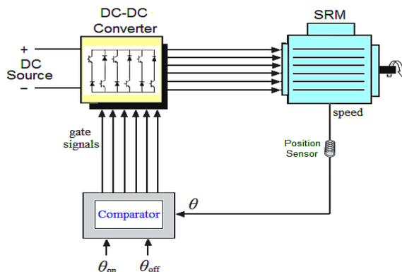
Fig. 1 Three-ph 6/4 SRM drive system
