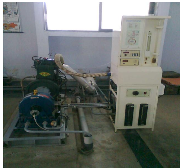
Fig.1 Single Cylinder 4-Stroke Diesel Engine Test Rig
