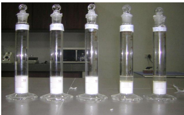
Figure 2: Photograph of slurries taken for sedimentation study (left to right 0%PE, 0.25%PE, 0.50%PE, 0.75%PE, and 1.0% PE respectively)
