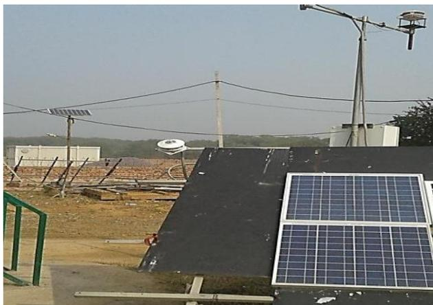
**Fig.1** PV modules of **Reliance** and **Waaree** in outdoor exposure
