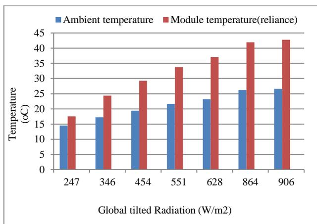
**Fig.4** Variation of Global Tilted Radiation (W/m<sup>2</sup>) with ambient and module temperature (°C) respectively for RS 1250 Reliance multi- C-Si PV module
