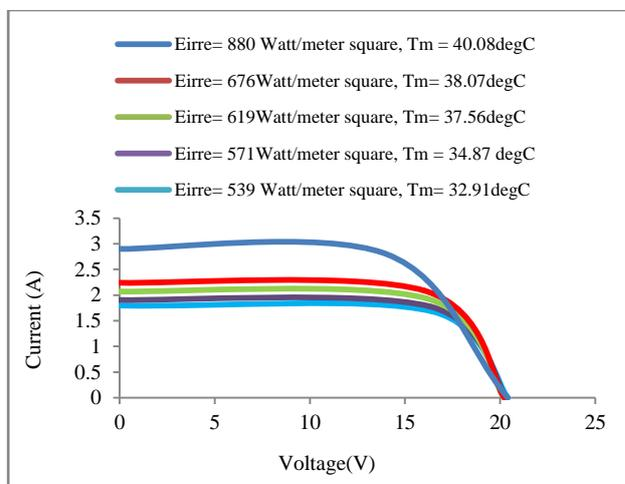
**Fig.6**WS-50(Waaree) PV module I-V characteristics in outdoor testing
