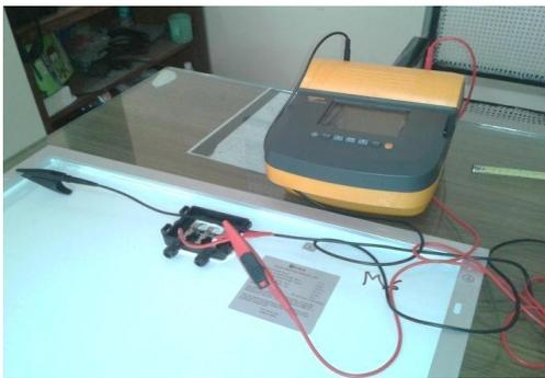
The test is performed by using Insulation Tester of FLUKE Company of model no 1550C/1555 for DC insulation testing with a current limitation. For modules with an area of less than 0.1m<sup>2</sup> the insulation resistance shall not be less than 400MΩ, for modules with an area of more than 0.1m<sup>2</sup> the insulation resistance times the area of the module shall not be less than 40MΩ m<sup>2</sup>.
