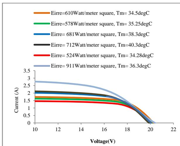
**Fig.7** RS-1250 (Reliance) PV module I-V characteristics in outdoor testing
