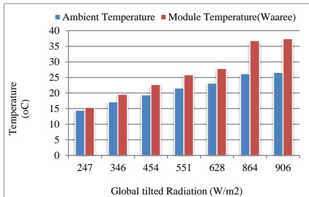
**Fig.4** Variation of Global tilted Radiation (W/m<sup>2</sup>) with ambient and module temperature (°C) respectively for WS 50 Waaree multi- C-Si PV module
