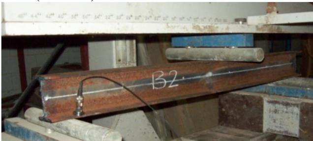
Figure (2) Experimental Test Rig of Mid Span Cracked Beam in Second Phase Boundary Condition (Hinge-roller)
