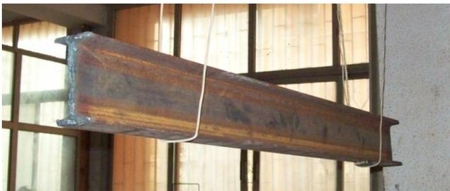
Figure (1) Experimental Test Rig of Intact Beam in First Phase (Free-Free)
