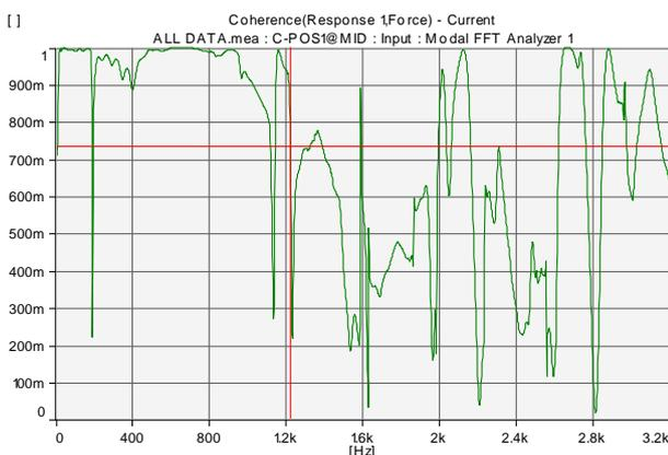
**Figure (7. b)** Coherence in Intact Beam in Case of Boundary Condition
