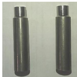
Figure 2: Titanium Alloy Ti-6AL-4V before EDM machining
