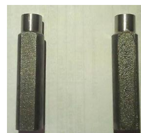
Figure 3: Titanium Alloy Ti-6AL-4V after EDM machining
