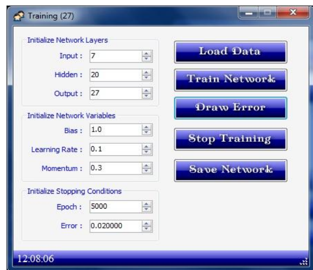
Fig 3: window of parameters used for designing and training BPNN.
