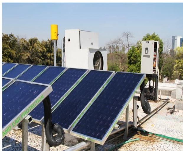
Fig. 2 Experimental Demonstration of Evacuated Flat Plate Collector at SEC
