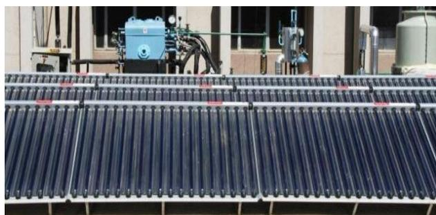
**Fig. 4** Experimental Demonstration of 1.5x Non Imaging Concentrator Collector or Compound Parabolic Concentrator Collector at SEC
