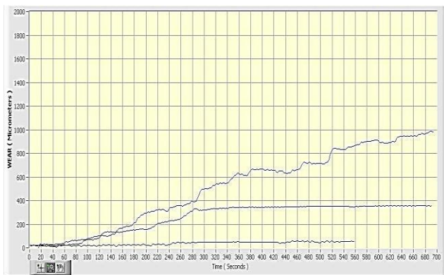
Fig 3 –Wear behaviour of MMCS with different % of Fly ash at 20N load and 240rpm.
