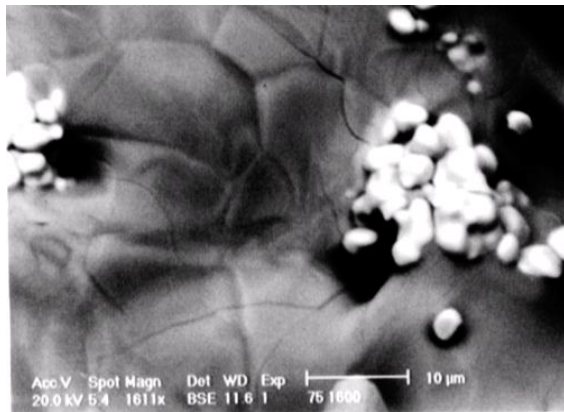
Figure 10 SEM micrographs of the TCP-ZrO 2 composites sintered for one hour at various temperatures with different percentages of TCP : (a) 25 wt%, 1500 °C; (b) 25 wt%, 1600 °C; (c) 50 wt%, 1500 °C; (d) 50 wt%, 1600 °C; (e) 75 wt%, 1500 °C and (f) 75 wt%, 1600 °C.
