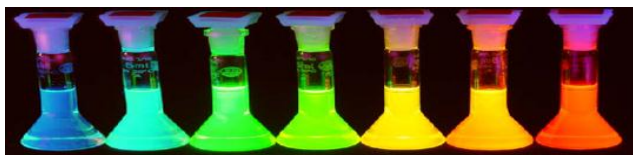
Figure 7 Size dependent multicolor emission of Quantum Dots
