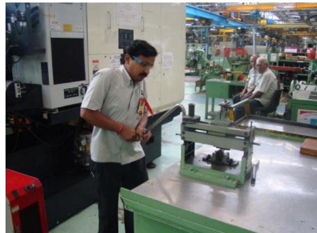
Fig.2 Manual punching operation – stresses in whole body
