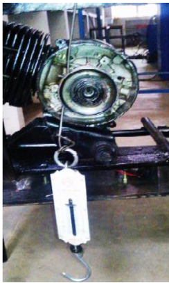
Fig.17: Brake Drum and Spring Balance Assembly
