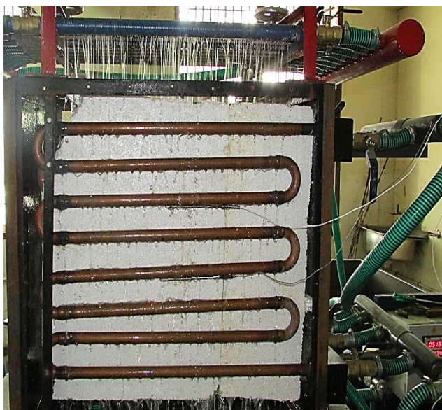
Fig.1 Photographic view of a row of horizontal tubes used in the experiments with cooling water droplets falling off the tubes
